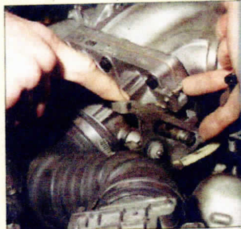
The throttle stop and roller bearing linkage are important factors when tuning this engine.
