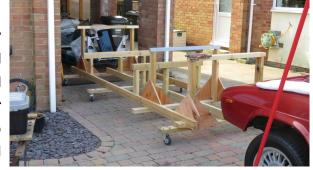
air however why did the body keep swinging to "port". Because I didn't undo the two earth cables on that side, one to the chassis and the other to the battery. Once sorted the lift continued and the rolling chassis pulled out from underneath the body.
