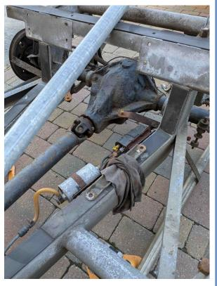
swinging arm housings to be very religious, (extremely holy!). Hmmm, a plan B was called for. A phone call to the ever-helpful Nigel at QRG. resulted in rear axle heading for Kettering for Nigel and his team to work their magic, replacing swinging arm housings and overhauling the whole thing.
