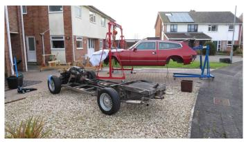
Old chassis now attacked big time at the rear, with many more ceased and rusted nuts & bolts cut off or induction heated off, all holding the back axle, anti roll bar and anti tramp mechanisms in place. Soon after, the rear swinging arms were off, soaked in my electrolytic bath to move rust followed by much fun braking up the old rubber bushes, sleeves, etc. then fitting nice new shiny poly bushes, plus
