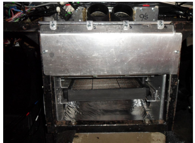
New Heater Box Showing Larger Matrix In Situ
