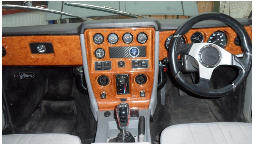
MB50's New Dash Showing the Revised Ducting Either Side of the Console
