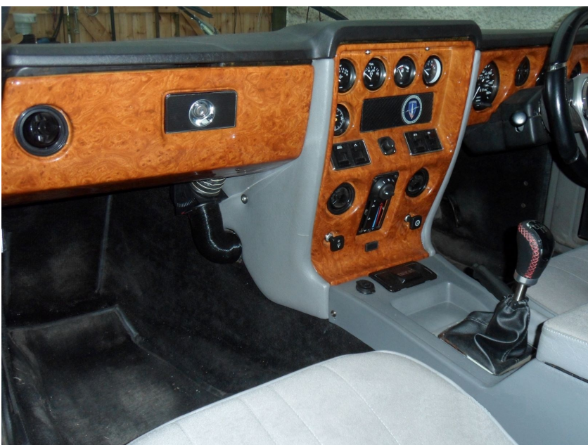
New Ducting and Diverter Valve with "Quick Release" Side Panels
