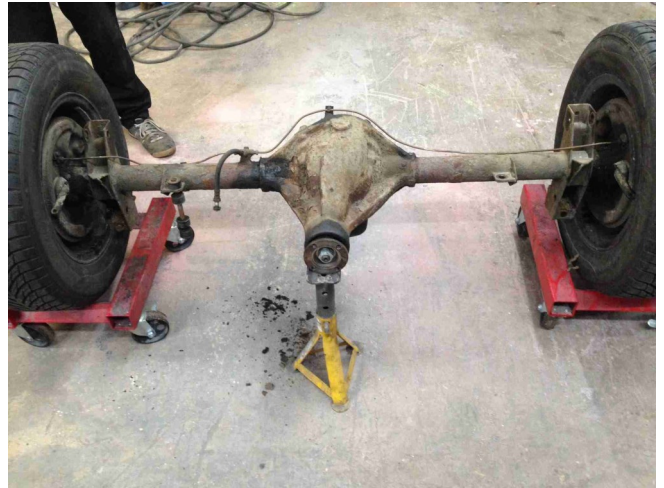
The Axle as Removed from Middlebridge 33
