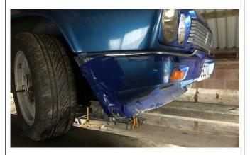
• Removing the rear bumper was not a pleasant job necessitating removal of the inner trim panels, all but one of the fixings had to be cut off. The fact that the rear section of the front bumper was missing helped with access for a grinder, it still took 8 or so hours.
