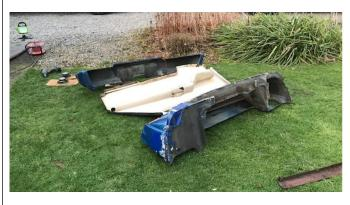
Going forward I have the bumpers to repair, the front is a challenge as much of the front scoop edge will have to be cut away and replaced to get remove the stress cracks, and the rear section modelled and probably a mould made. The rear has a couple of areas that need grinding out but nowhere near as much effort required.
