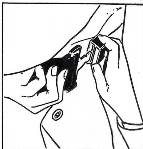
Figure 4 — Rear seat belt lap strap engagement
